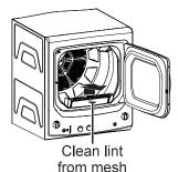
**Dryer Interior and Duct:** The interior of the appliance and exhaust duct should be cleaned once a year by qualified service personnel.
